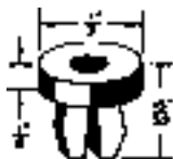
N-164P (3783006) Screw Size #8 Panel Hole .280" sq. Panel Range .031-.156"
