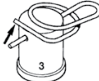
TO REMOVE PUSH UP AND BACK ON CAM RAMP
