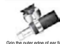
Grip the outer edge of ear firmly and cut through it with either pincers.
