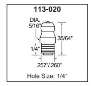
Drive type fittings are designed for fast production line installation in untapped holes, to avoid thread tapping costs. The hole sizes and shank dimensions are for reference use only. Test applications should be conducted to determine the correct hole size, which varies
