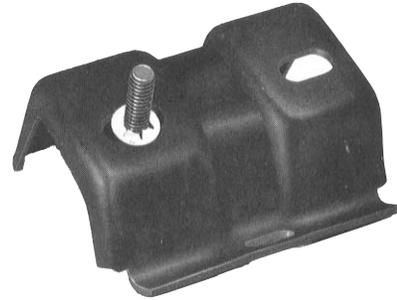
Style PT Retainer, above, retains carriage bolts in slots in this auto bumper bracket until the bumper itself is attached by running down a hex nut.
